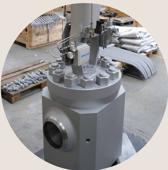
Fig. 10. Feed water control valve for conventional power plant. Angle forged type of 8" class 2500# with an operation pressure drop of 300barg.
