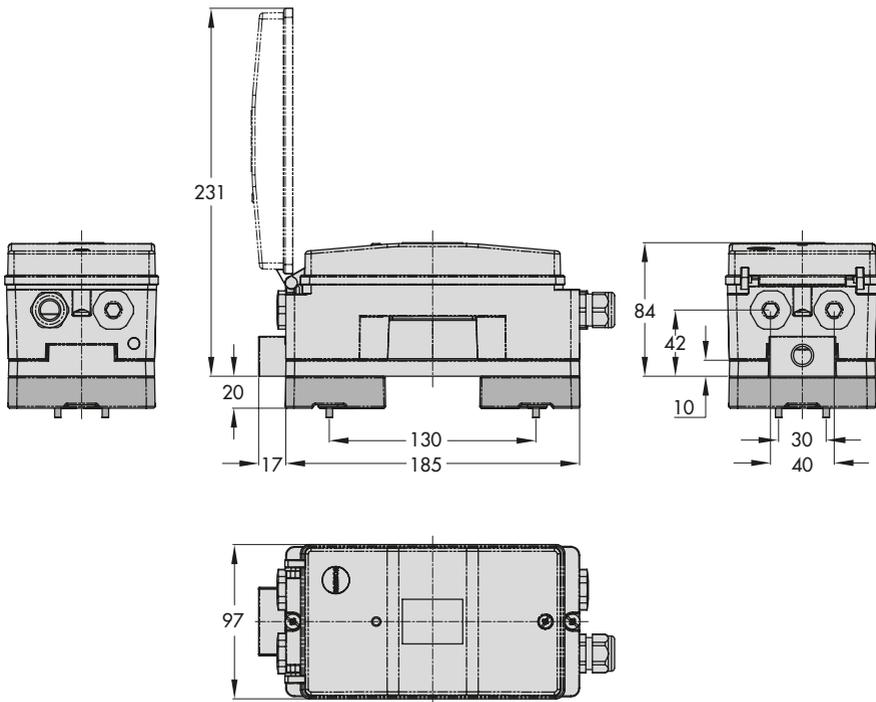
Attachment to linear actuators according to IEC 60534-6 (NAMUR)
