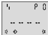
**P0:** Display when the electronic limit switch has not yet been initialized
