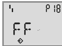
P18: FOUNDATION™ fieldbus write protection: NO
