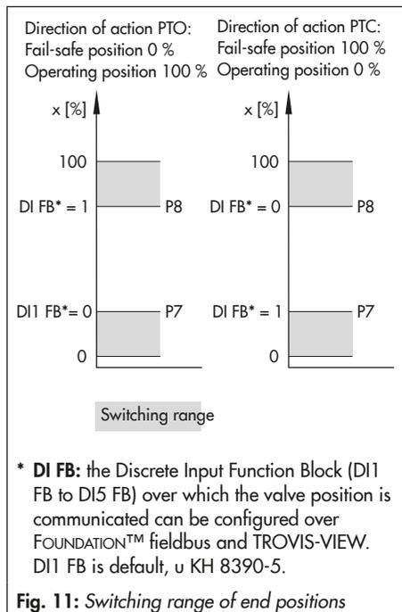
**Fig. 11:** Switching range of end positions
