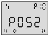
**P10:** Confirmation of operating position (solenoid valve energized)
