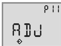
**P11:** Zero/end position calibration in progress
