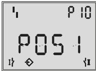
**P10:** Confirmation of fail-safe position (solenoid valve de-energized)
