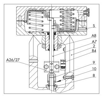
Fig. 12: Type 3271 Pneumatic Actuator on a Series 240 Valve
