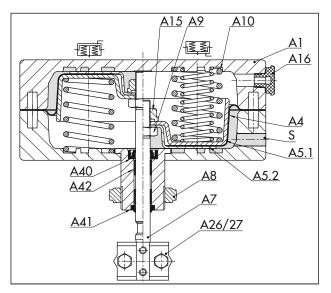
Fig. 2: Type 3271-5 Actuator, drawing showing an example with 120 cm<sup>2</sup> actuator area
