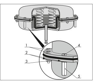
Fig. 22: Preloaded springs (functional diagram)
