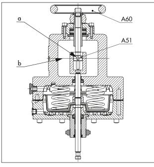
Fig. 17: Type 3271-5 Actuator with handwheel
