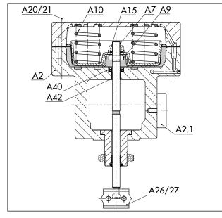
Fig. 4: Type 3277-5 Actuator with 120 cm<sup>2</sup> actuator area
