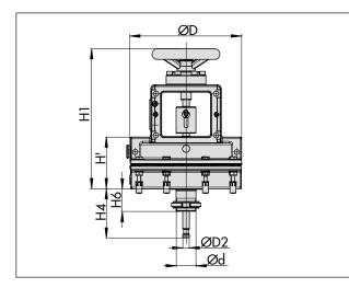
Fig. 8: Type 3271-5 with additional handwheel
