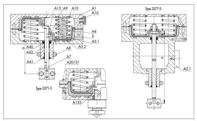
Fig. 18: Type 3271-5 and Type 3277-5 Pneumatic Actuators
