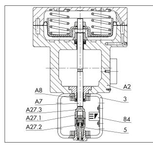
**Fig. 21:** Type 3277 Pneumatic Actuator on a Type 3510 Micro-flow Valve
