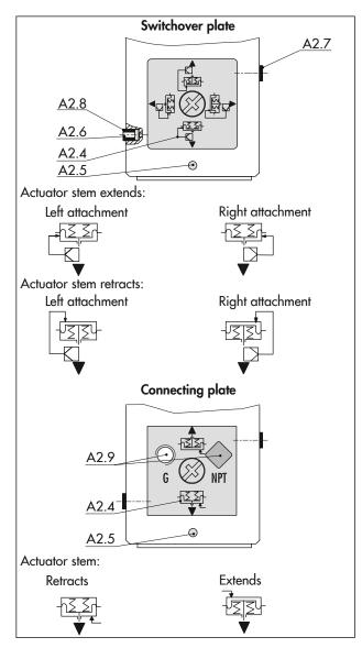
**Fig. 15:** Switchover plate and connecting plate on Type 3277-5
