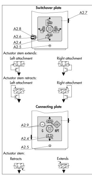
Fig. 6: Switchover plate and connecting plate on Type 3277-5
