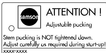
Fig. 2: Label when an adjustable packing is installed
