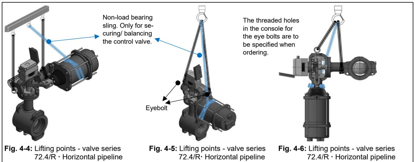
**Example for lifting the valves Type 82 with actuator Type R**
