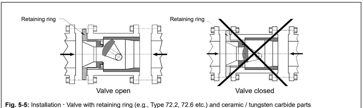
To ensure tightness to the atmosphere, cover the area between the armoured sleeve (e.g. made of ceramic or hard metal) and the valve body with the sealing surface of the pipeline flange. See Fig. 5-6 / Table 5-3.
