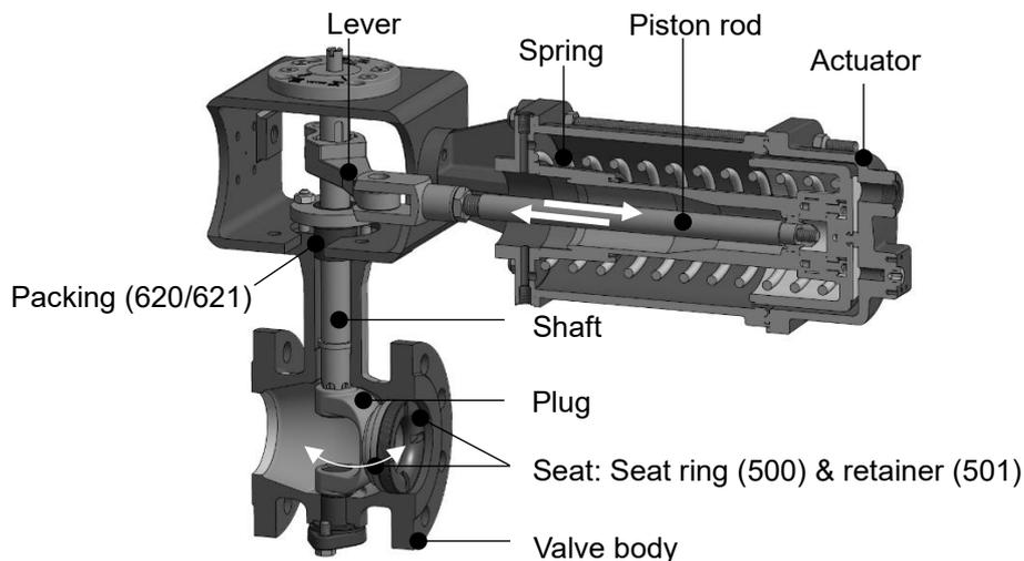
**Fig. 3-22:** Rotary plug valve with actuator Type R · Principle of operation
