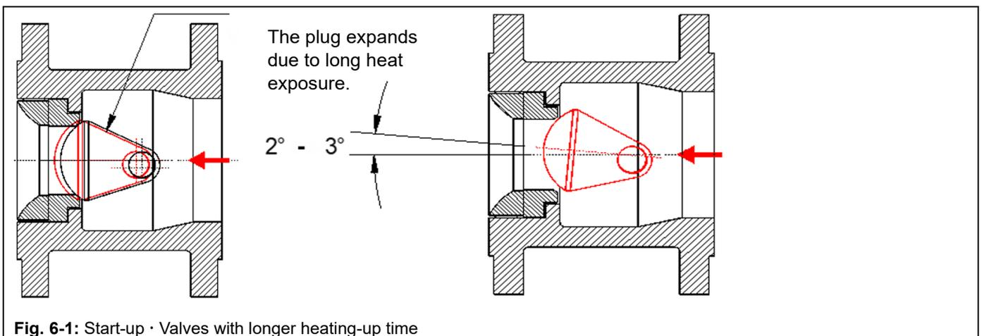
Fig. 6-1: Start-up · Valves with longer heating-up time
