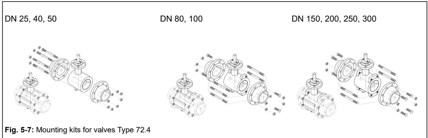
Fig. 5-7: Mounting kits for valves Type 72.4
