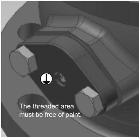
**Fig. 5-1:** Ground connection Valve Type 72, 73, 82
