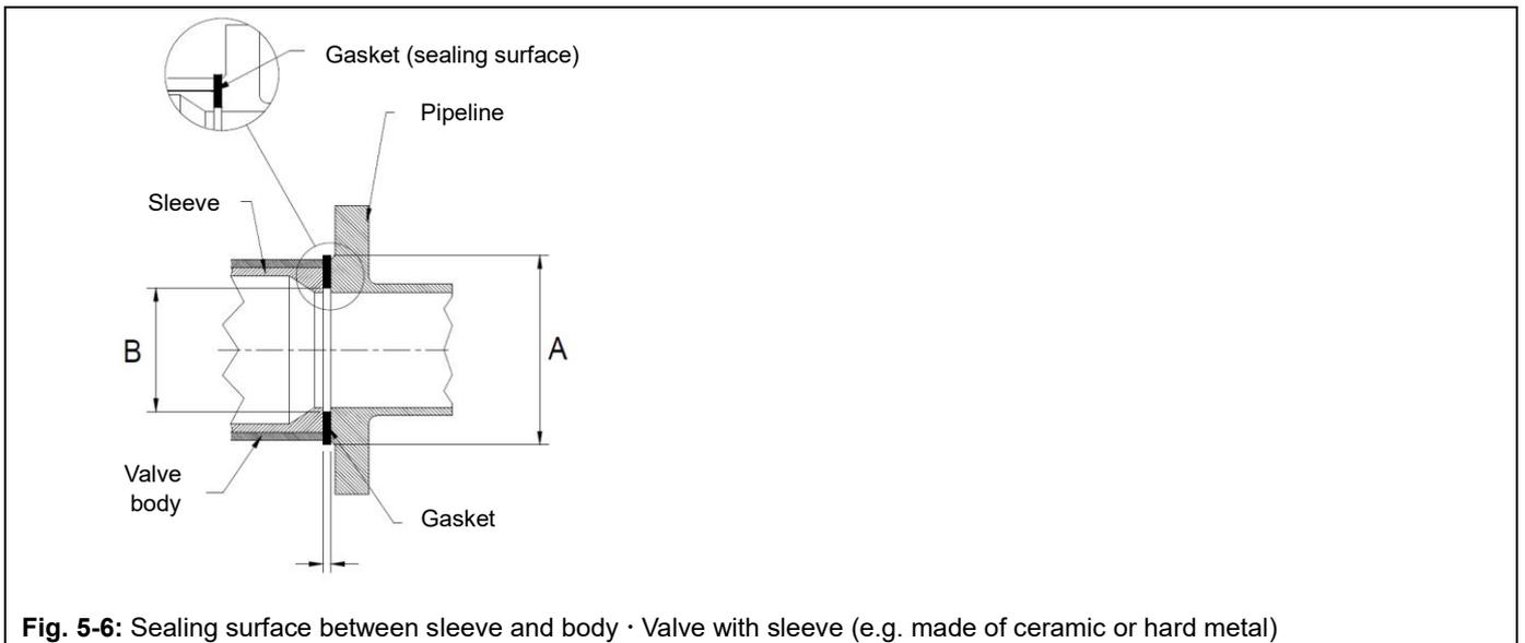
**Fig. 5-6:** Sealing surface between sleeve and body · Valve with sleeve (e.g. made of ceramic or hard metal)
